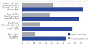
Slip Resistance Test EN ISO 13287:2012, performed by TUV Rheinland LGA Products GmbH in Leipzig, Germany during August 2018\* On a scale where 0.0 is the absence of friction and 1.0 is very high riction (e.g. dry carpet), SFC rated. 83 – more than tripling the .18 minimum standard. All SFC shoes use the Shoes For Crews patented slip-resistant outsole. Product tested:SRIDGETOWN 28740
