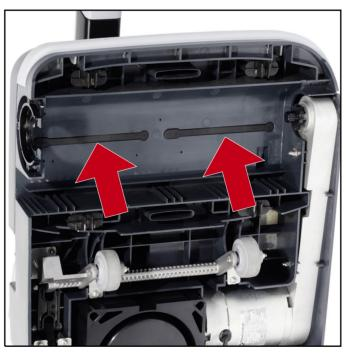
3. Check if the holes in solution dispensers are clogged. Remove them and clean if needed.
