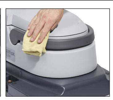
16. Clean the machine using a damp cloth and where needed use a neutral cleaning product.
