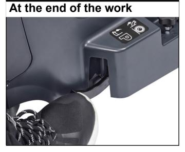
11. For the transportation and the parking of the machine, push down the pedal (slightly lift the front of the machine by tilting the handlebar).
