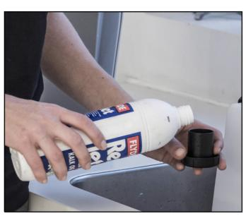
3. The tank cap can be used for dosing the detergent. One full cap is 30ml giving 0,5% detergent of the 6L tank capacity. (\*)
