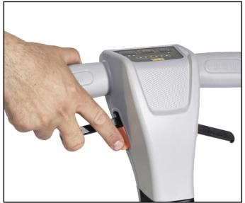
right lever to lift the front squeegee in order to collect light debris.
