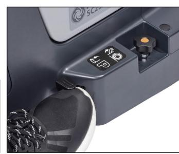
5. Lift the pedal to lower the machine and start working.
